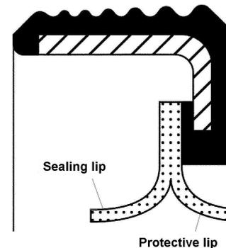
The material polytetrafluorethylene (PTFE), however, provides a solution. PTFE oil seals do withstand these extreme stresses since they
