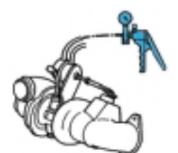
Checking the discharge valve of turbo engines
