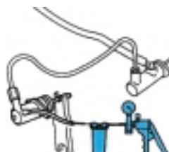
Draining out the coupling fluid
