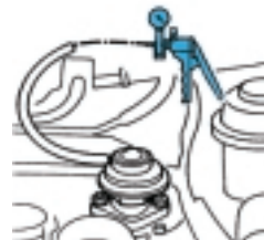
Checking the exhaust gas return (EGR)
