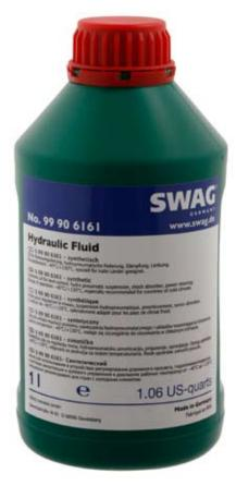
SWAG 99 90 6161 Central Hydraulic Oil (synthetic) was developed for use in systems for the central hydraulics/level control/ hydropneumatic suspension, as well as damping and steering in the range of use from -40°C to +130°C.
